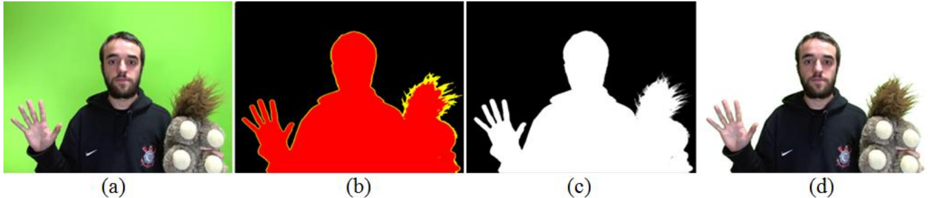
Figure 2: (a) RGB picture. (b) Trimap – foreground (red), background (black), “unknown” (yellow). (c) Alpha map. (d) Composite image.
