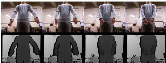
Fig. 2. Input data is a video sequence of one texture and one depth map images per frame. The texture image provides RGB values while the depth map image gives us triplets (x, y, z) .
