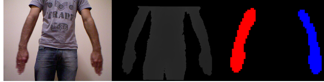
Fig. 1. Detection and segmentation of movement (right) using our method applied to texture (left) and depth (middle) images. Red and blue colors indicate movement to right and to left, respectively.
