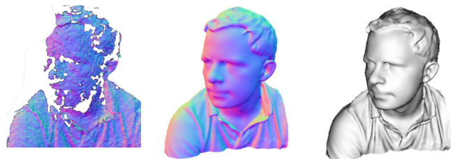
Fig. 7. Data with noise and hole filtered with KinectFusion technique.
