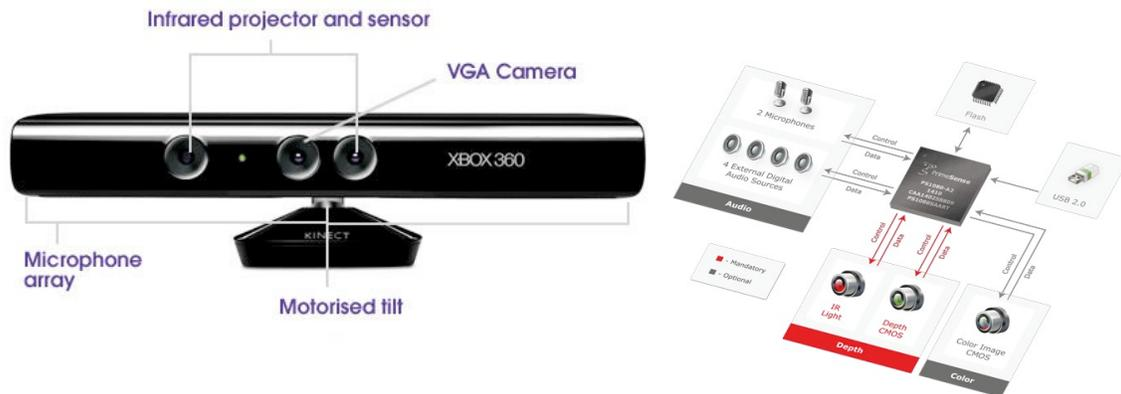
Figure 3.1: Kinect device and chip.
