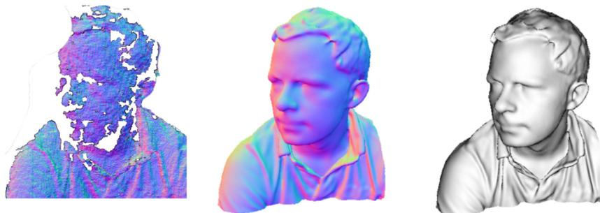
Figure 4.3: Data with noise and hole filtered with KinectFusion technique.
