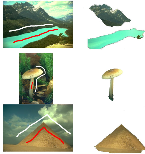
Fig. 9. Original images with chosen seeds (red marks: foreground seeds, white marks: background seeds) and GrabCut segmented images. Accuracy rates (compared to ground truth of Figure 7) for the 3 images are, respectively, 73.94%, 95.71%, 91.09%.
