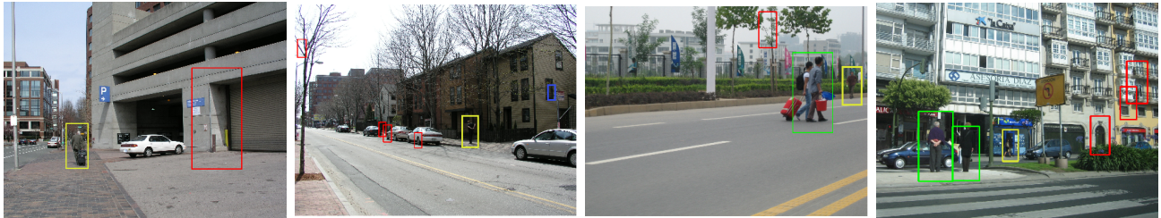
Fig. 12. MSR negative results at 30% of WSR after non-max suppression. Yellow rectangles indicate FN caused by MSR (affecting performance); blue rectangles indicate avoided false positives (improving performance); TP are marked with green, while red rectangles are FP.
