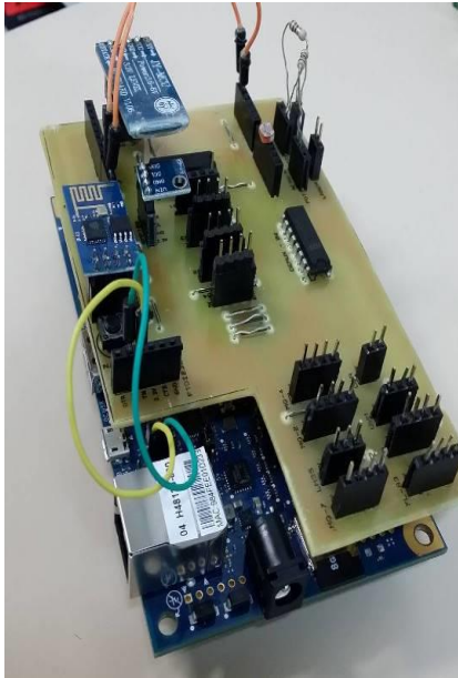
← Passive Sensor Board (PSB) with 14 Sensors connected
