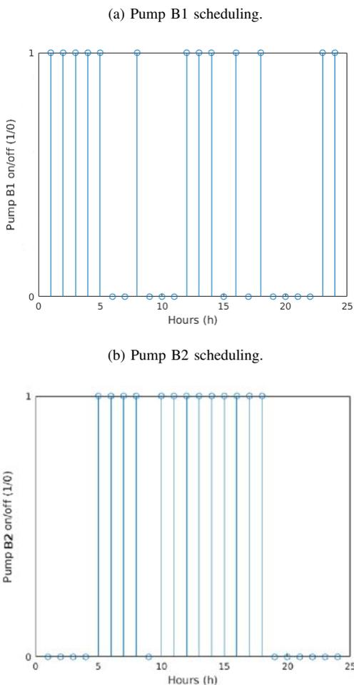
To better understand the scenario, the daily total pumping cost, using the schedule presented by Figure 11 and the Brazilian seasonal green price of electric power, reaches R\$34.89. When using a bang-bang control scheme with a simple logic
