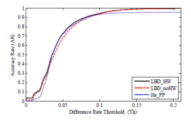
Accuracy rate vs. difference rate threshold on CASIA-Iris-Thousand database
