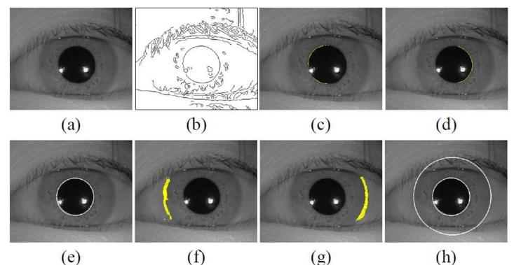
(a) Original Iris (b)Canny edge image; (c), (d), (f), (g) Yellow pixels are detected by learned left pupillary, right pupillary, left limbic and right limbic boundary detectors respectively; (e), (h) Pupillary and limbic boundaries fitted as circles by weighted Hough transforms.
