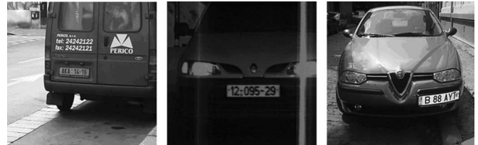
Fig. 10. Images from test sample 5. The one in the middle was captured using infrared illuminator and special camera for night operation.
