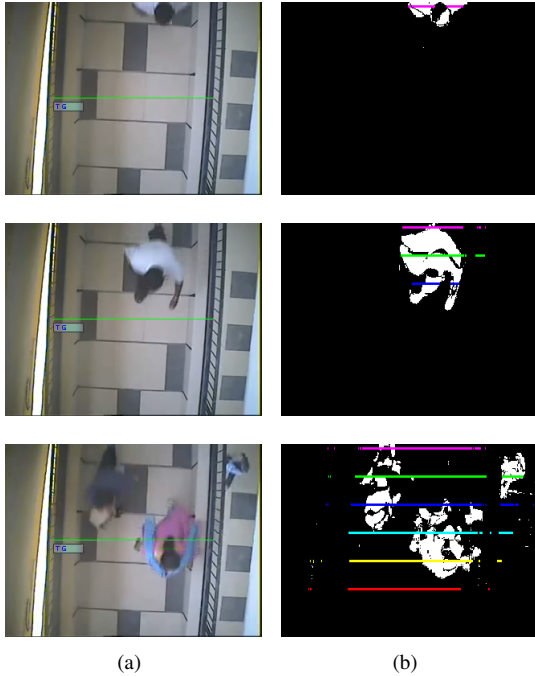
Figura 5. Results showing the steps of multiple lines. (a) original frame. (b) frame segmented and with lines.
