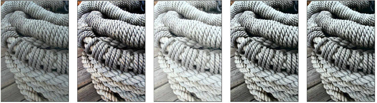
Figure 195: Results for the "138032.png" image: (a) original image; (b) C1DHE ; (c) TV3DHE ; (d) our HP1DHE ; (e) our HP2DHE .
