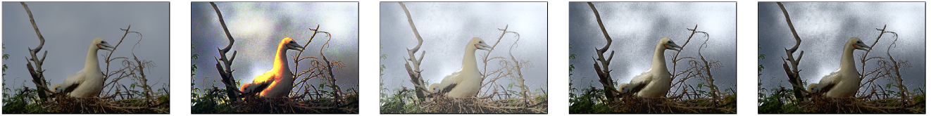
Figure 196: Results for the "8049.png" image: (a) original image; (b) C1DHE ; (c) TV3DHE ; (d) our HP1DHE ; (e) our HP2DHE .
