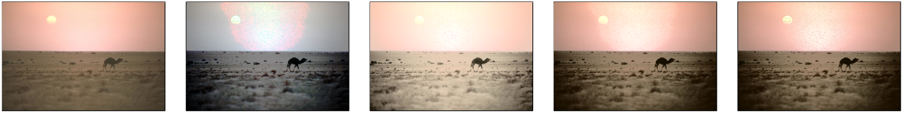
Figure 188: Results for the "271031.png" image: (a) original image; (b) C1DHE ; (c) TV3DHE ; (d) our HP1DHE ; (e) our HP2DHE .
