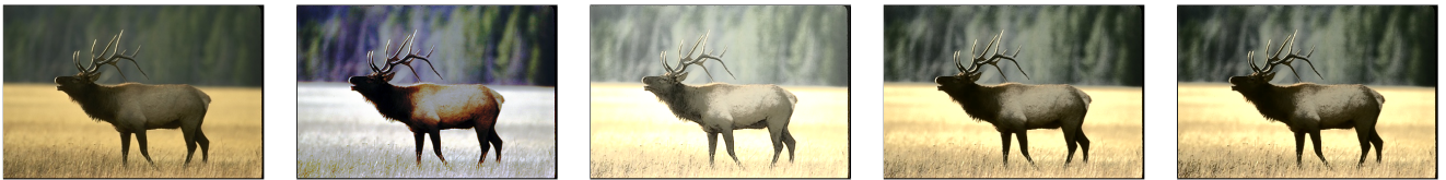
Figure 33: Results for the "41004.png" image: (a) original image; (b) C1DHE; (c) TV3DHE; (d) our HP1DHE; (e) our HP2DHE.
